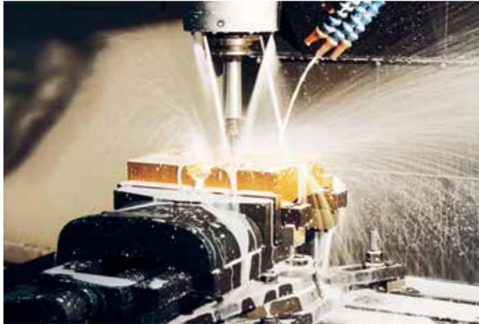
80% of the machining procedure done at one setting due to efficient computerized programming and large pool of the tool magazine.
